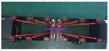
Step 2: Lock M3\*5 cross countersunk head screw in the position as the the red arrow pointed in the following pic.
