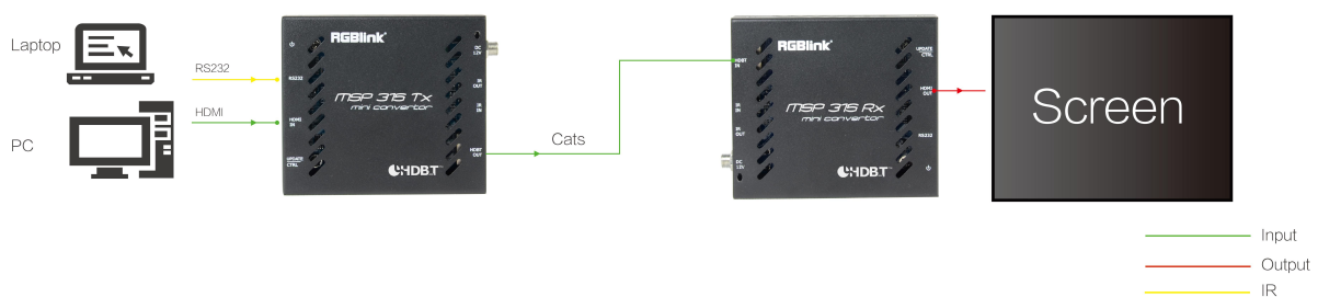
MSP 315 HDMI Extender System Connection Diagram
