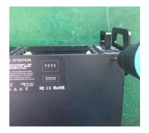
Step: Clean dust on the front and back of the fan module by brush.
